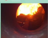
Automatically supplied into the ARC continuously, the rice-husk turns into the regular charcoal w ithin 10 min.
