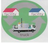
One portable type sludge dewaterer and dryer can treat some sewage water treatment facilities. Thus you don't have to transport sludge, and you can reduce cost. Power generator can be loaded, so each facility doesn't require power supply.
